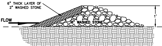
ROCK CHECK DAM DETAIL
