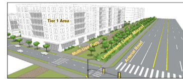
Figure 7: Illustration showing the landscaped linear mound, with placement of trees and other vegetation forming a buffer between the arterial road (on the right of the figure) and the Tier 1 area (buildings).
