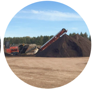
Finished compost is screened once before it is sold, removing larger particles that remain.
