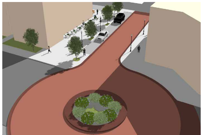
Overview of traffic circle with decorative pavers and planting bed.
