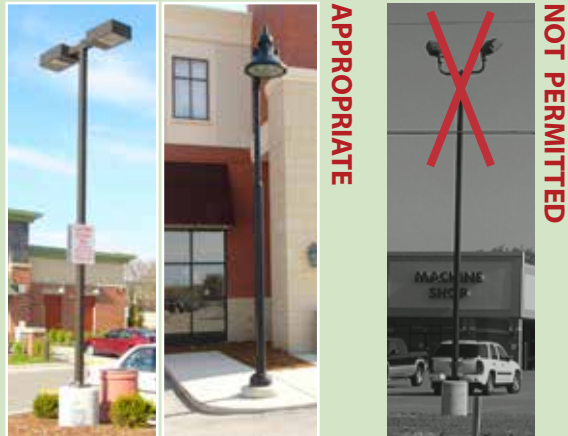
The two images on the left show good examples of low parking lot fixtures that project light only where it is needed, while the far right image shows an excessively tall light that is directed outward, creating glare and
