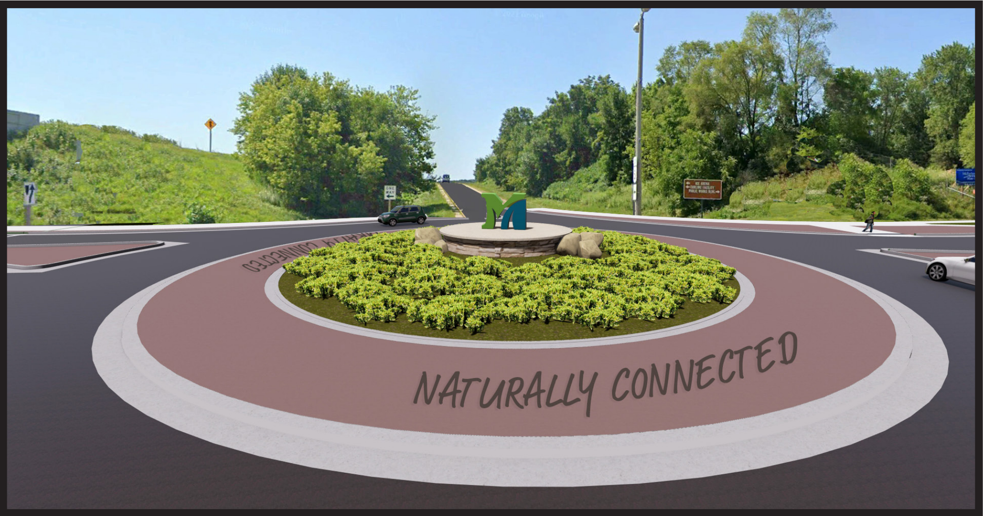
Short retaining wall with stone veneer, McFarland “M” logo and Rhus aromatica (fragrant sumac) or other ground cover plantings less than 30” tall.
