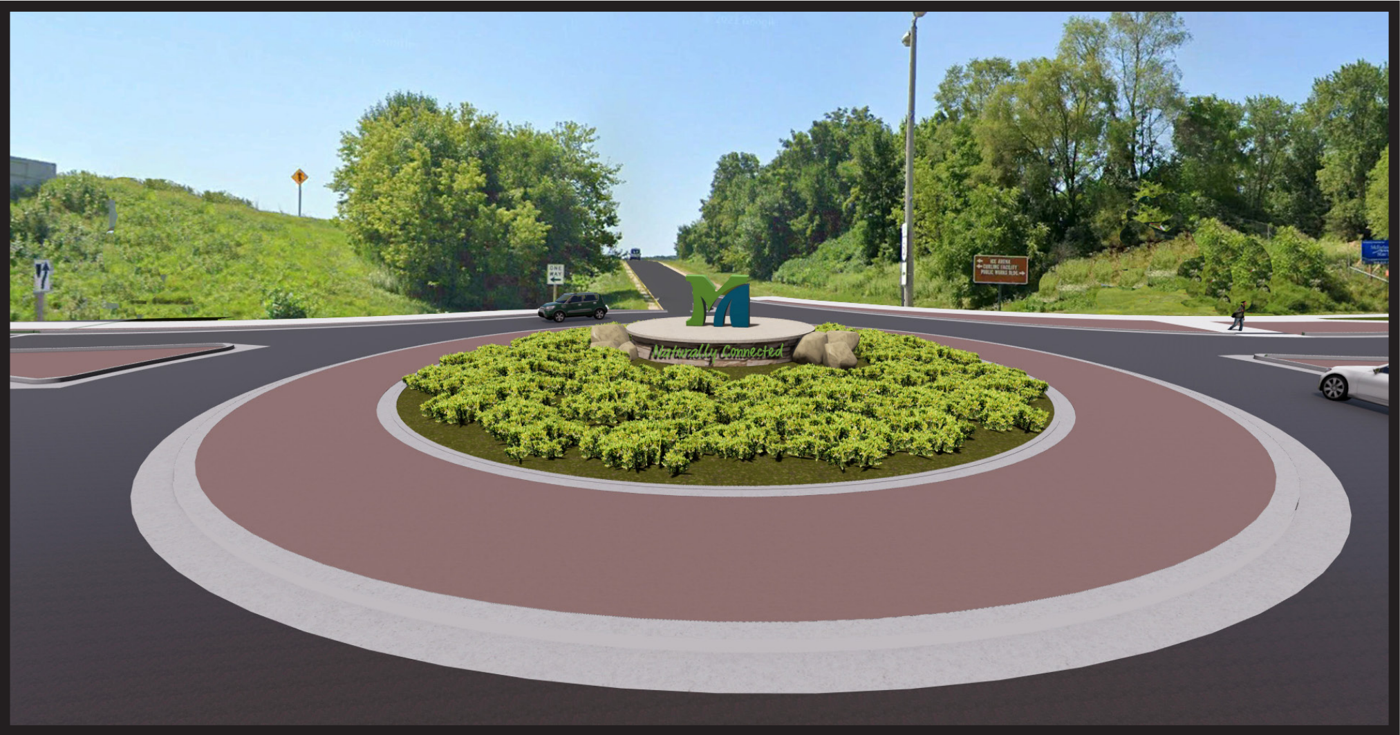
Short retaining wall with stone veneer, McFarland “M” logo and fragrant sumac ( Rhus aromatica ) or other short ground cover plantings.
