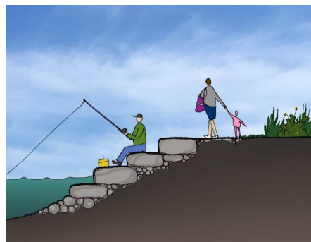
Stepped Stone Revetment Render
