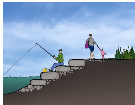
Stepped Stone Revetment Render
