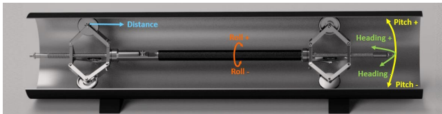
Figure 2: Pipeline 3D Data Collection
