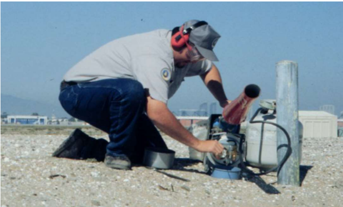
Figure 5. Gas-operated cannons, generally referred to as propane cannons, are commonly used to disperse geese, waterfowl, and coots.
