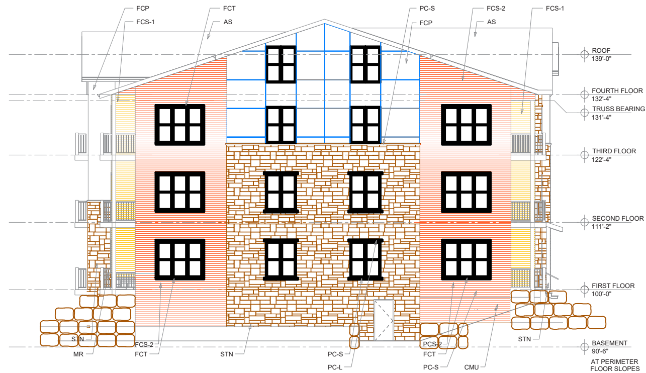
② SOUTH ELEVATION 1/8" = 1'-0" ON 22x34 HALF SCALE ON 11x17
