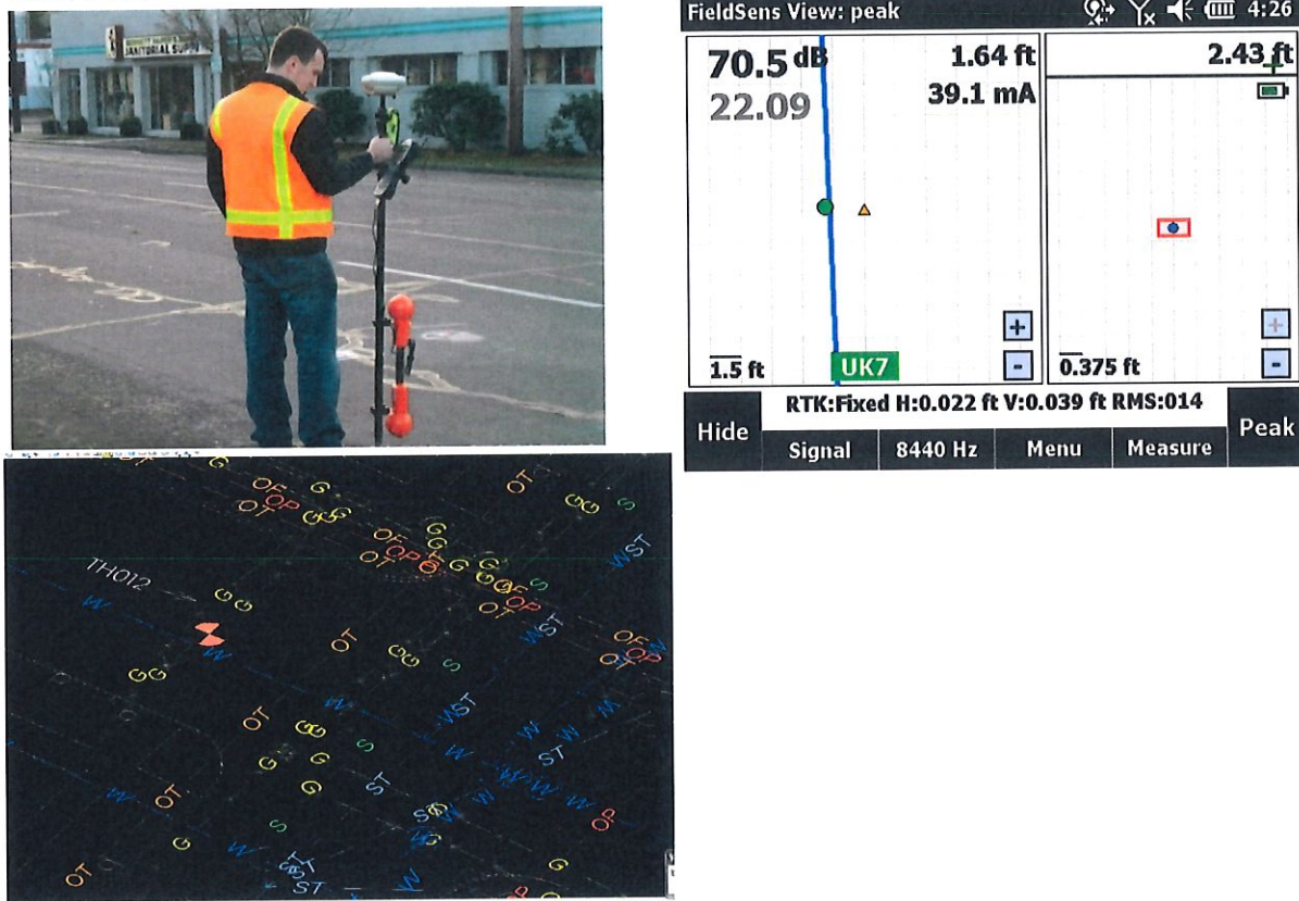
Figure 11. UMS uses GEOfeature™ to manage wide variety of acquired data which is merged to generate the 3-D GIS and CADD output products.
