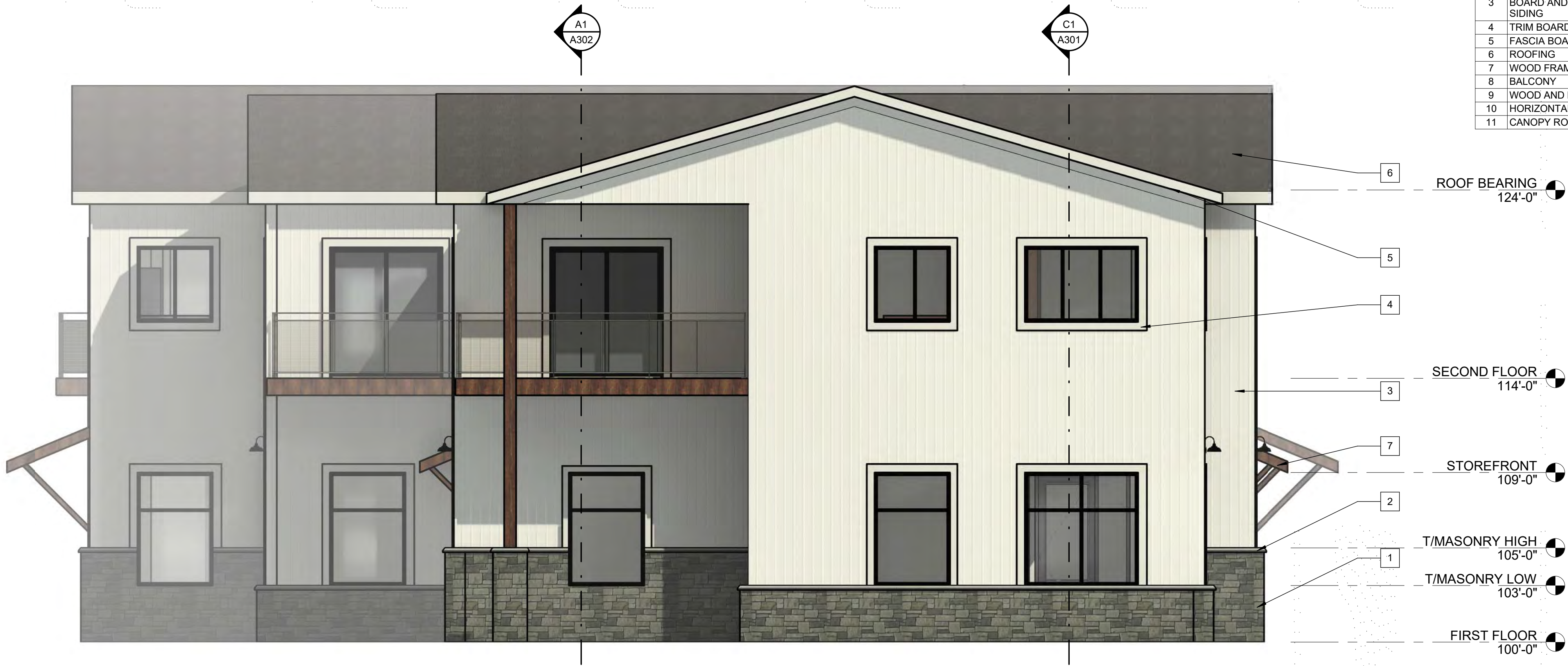
B1 NORTH ELEVATION 1/4" = 1'-0"
