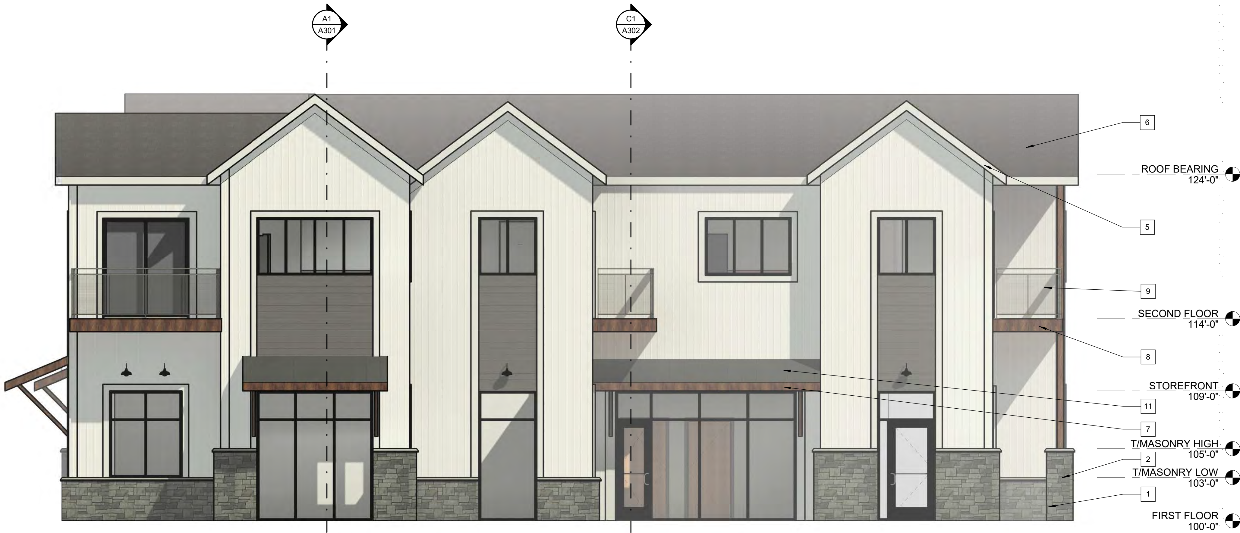
A1 EAST ELEVATION 1/4" = 1'-0"
