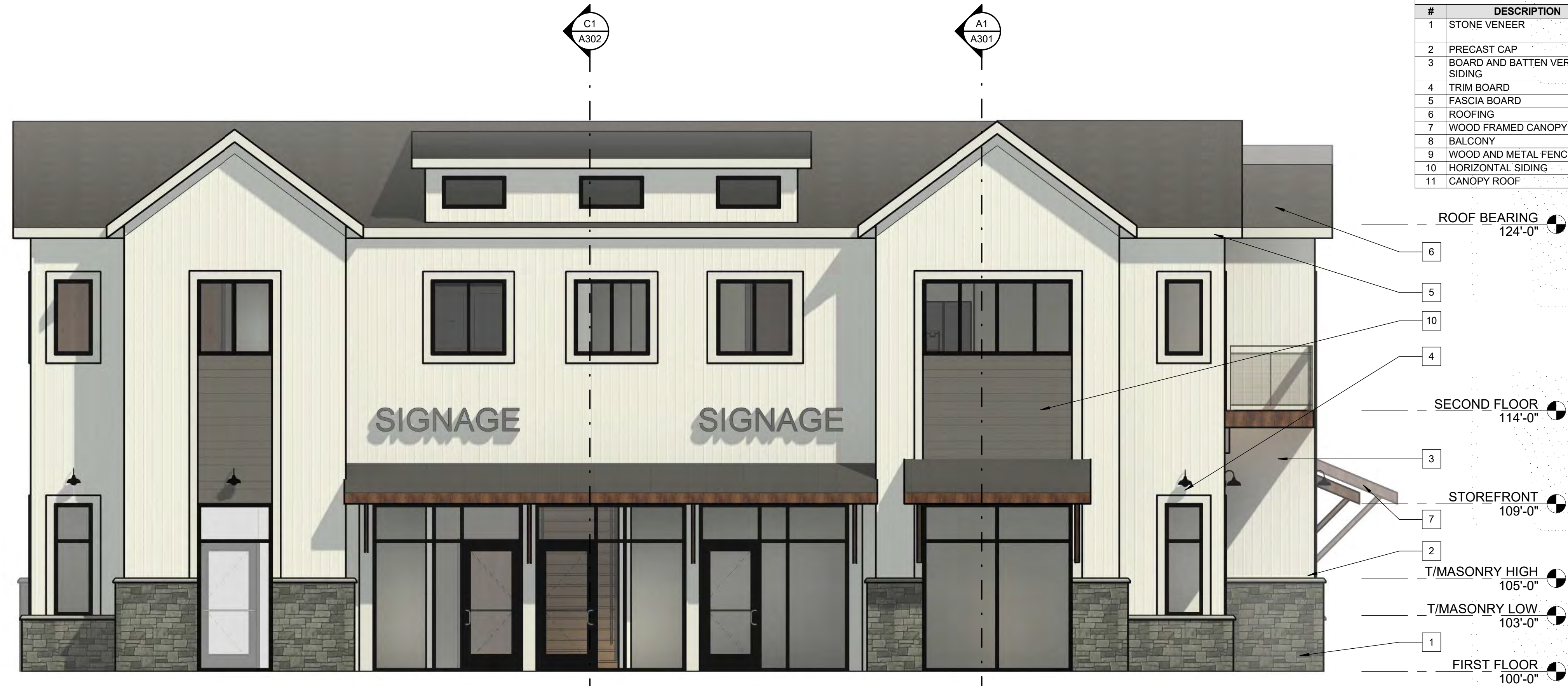
C1 WEST ELEVATION 1/4" = 1'-0"
